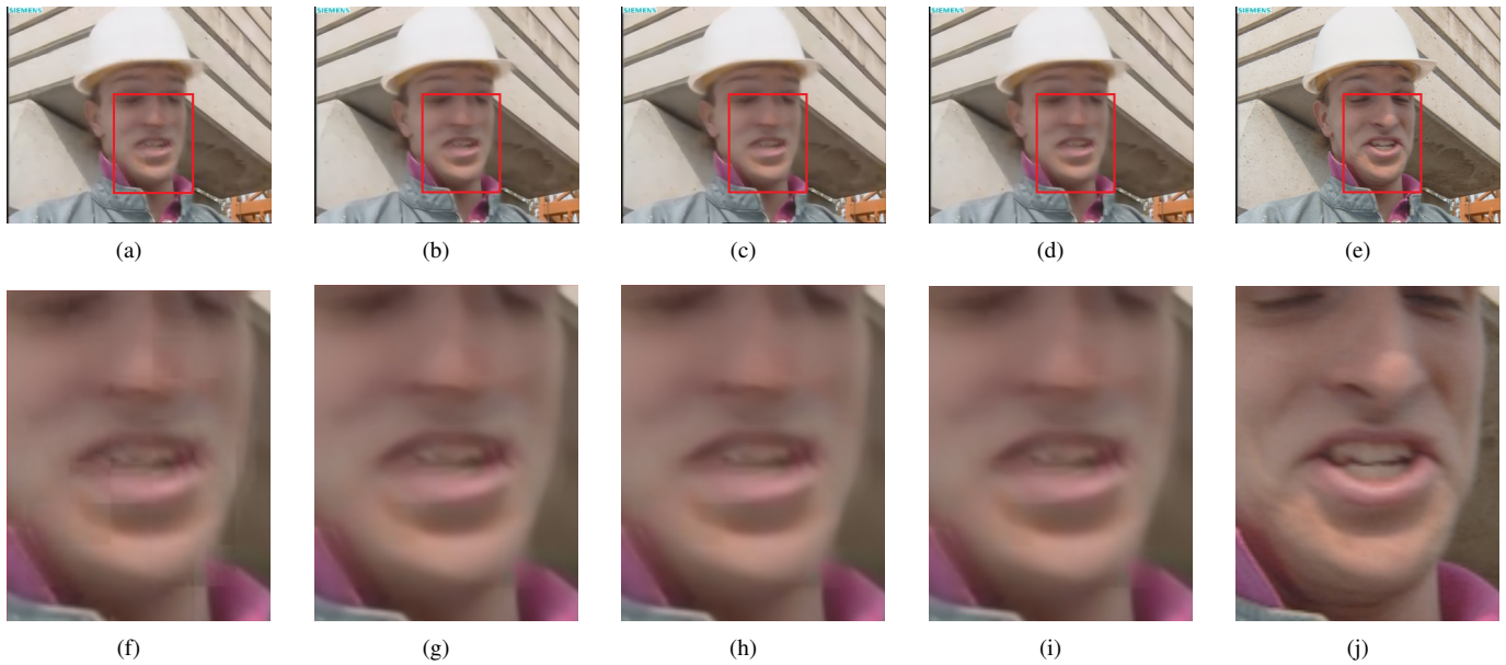
Fig. 8: The 79 th interpolated frames of Foreman reconstructed by different FRUC algorithms: (a) and (f) interpolated by DS-ME, (b) and (g) interpolated by DRNFRUC ( \beta = 0 ), (c) and (h) interpolated by DRNFRUC ( \beta = 0.005 ), (d) and (i) interpolated by DRNWCMC, (e) and (j) original image
